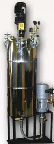
Agitated pressure tank with transfer pump
