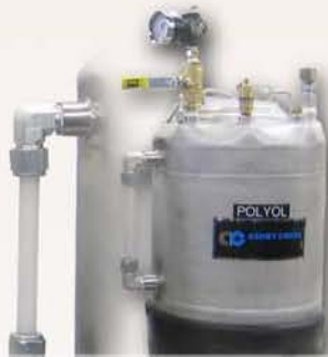
Sight tubes for visual level detection
