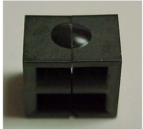
ECLIPSE 703 bridge bonding a ferrite core
