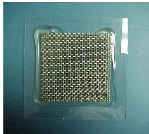
ECLIPSE 321 bonds metal to glass with a complete cure in the areas shadowed by the wire mesh.
